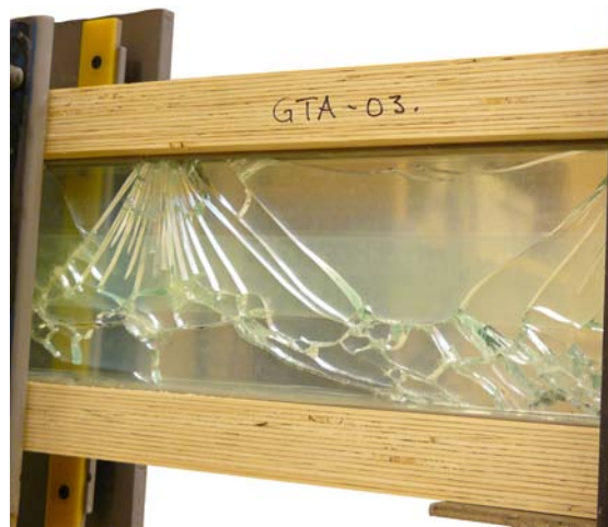
(b) Typical crack formation later in test (ALN-03).
