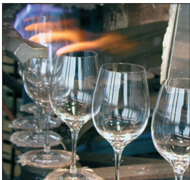
Figure 9.2 To ensure the edge is rounded, it is melted in an edge-melting machine. Sandvik.
