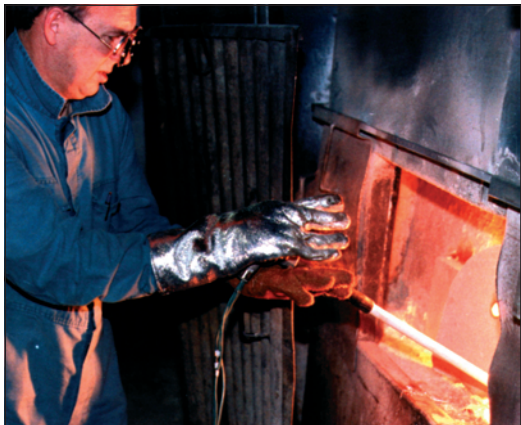
Figure 5.1 Measuring the temperature of the glass with a thermocouple in the form of an immersion pyrometer.
