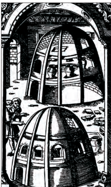
Figure 4.1 Agricola's round furnace from 1556.
