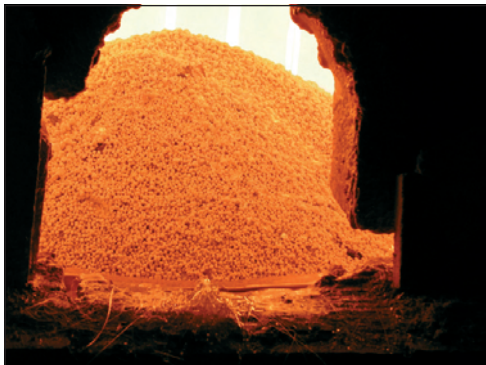
Figure 3.1 Pelletised batch that has been charged into the melting furnace.
