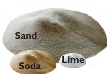
Figure 2.1 Raw materials of a soda glass.
