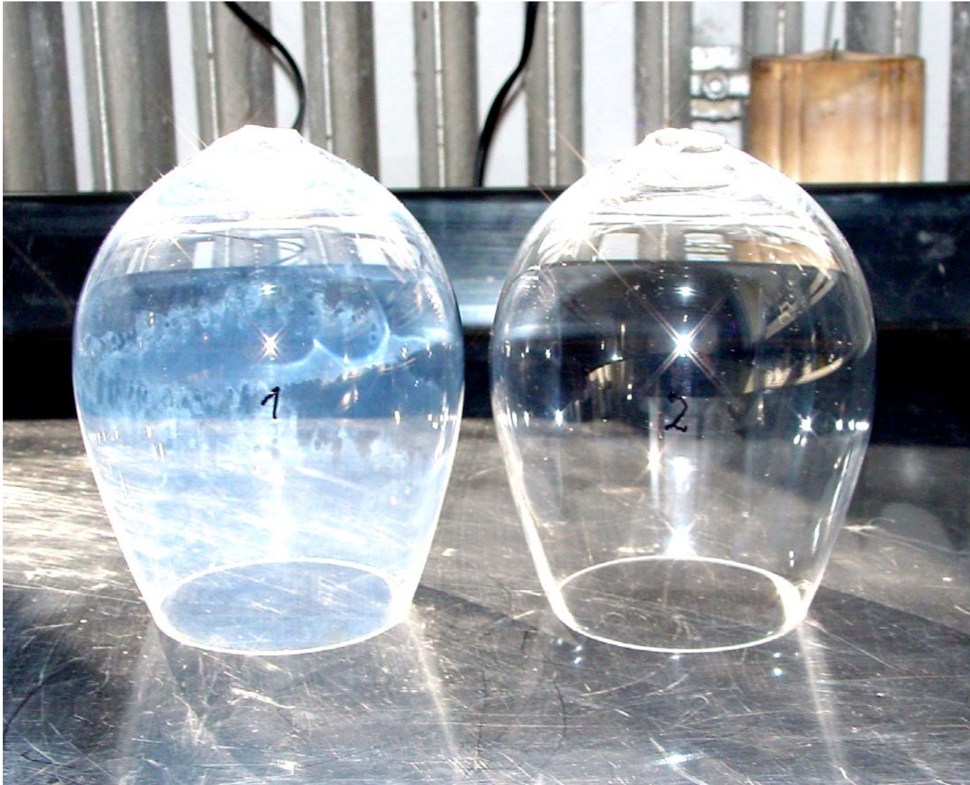
lead glass – after 72 hours immersion in distilled water at 90 °C; left: untreated; right: treated with \text{AlCl}_3
